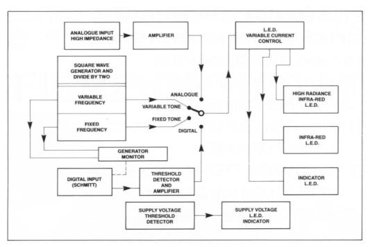
FIBRE-OPTICS MONITOR TRANSMITTER BLOCK DIAGRAM
